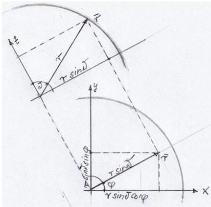
$$\begin{aligned}x &= r \sin \vartheta \cos \varphi \\y &= r \sin \vartheta \sin \varphi \\z &= r \cos \vartheta\end{aligned}$$
